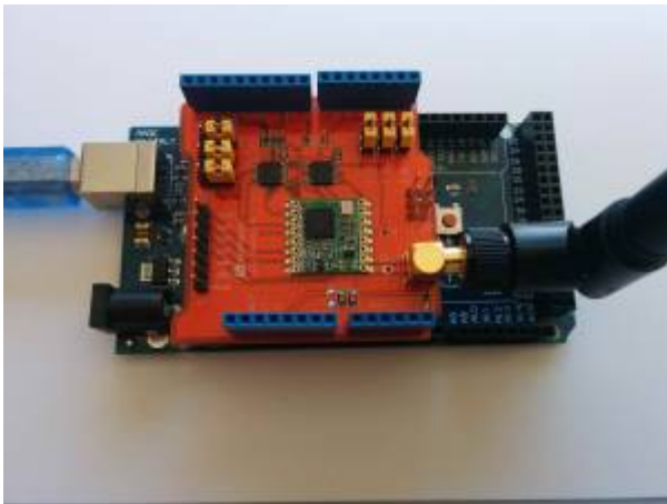
Figure 1. Arduino with LoRa Dragino shield.
