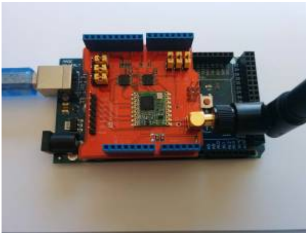
Figure 1. Arduino with LoRa Dragino shield.
