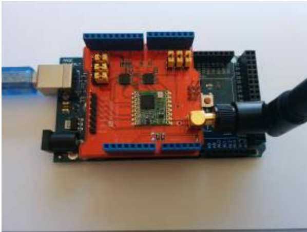
Figure 1. Arduino with LoRa Dragino shield.
