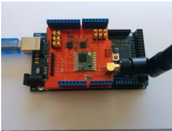
Figure 1. Arduino with LoRa Dragino shield.
