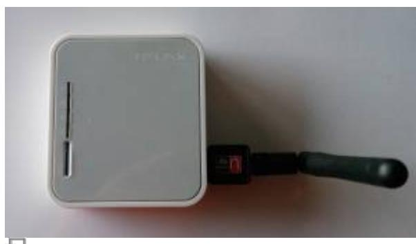
Figure 1. MR3020 with WLAN adapter
