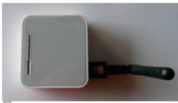
Figure 1. MR3020 with WLAN adapter
