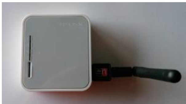
Figure 1. MR3020 with WLAN adapter
