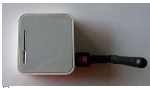
Figure 1. MR3020 with WLAN adapter
