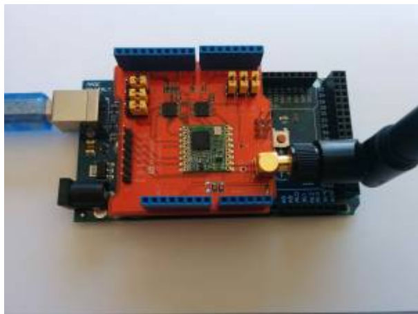
Figure 1. Arduino with LoRa Dragino shield.
