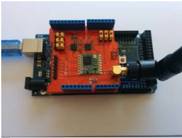
Figure 1. Arduino with LoRa Dragino shield.
