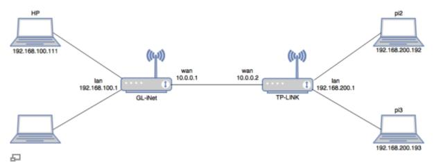
Figure 3. Addressing plan for QoS platform
