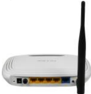
Figure 2. TP-Link WR741nd wireless router
