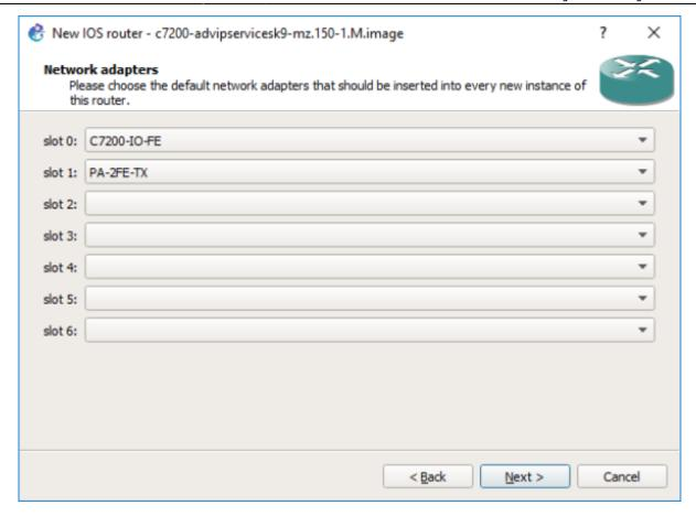
Apply to validate the new device parameters. Now you are set to start using Cisco routers with GNS3.
