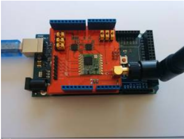
Figure 1. Arduino with LoRa Dragino shield.
