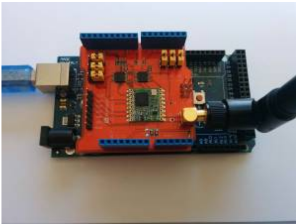
Figure 1. Arduino with LoRa Dragino shield.
