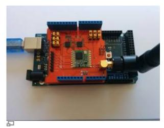
Figure 1. Arduino with LoRa Dragino shield.
