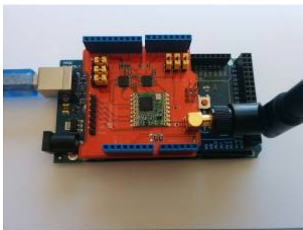
Figure 1. Arduino with LoRa Dragino shield.
