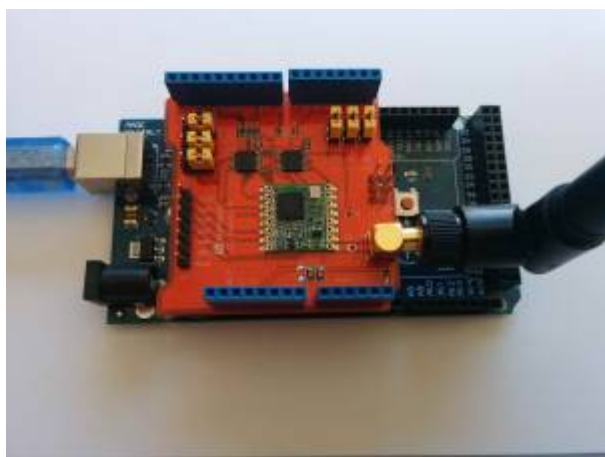
Figure 1. Arduino with LoRa Dragino shield.
