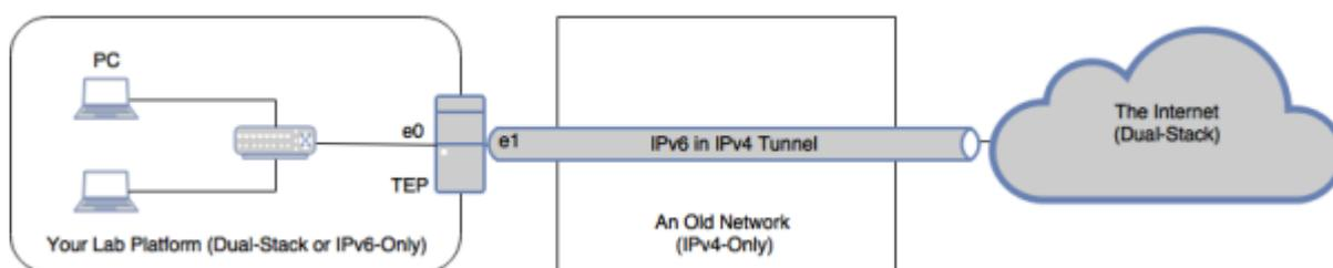
Figure 2. 6in4 Tunnel for extending IPv6 connectivity
