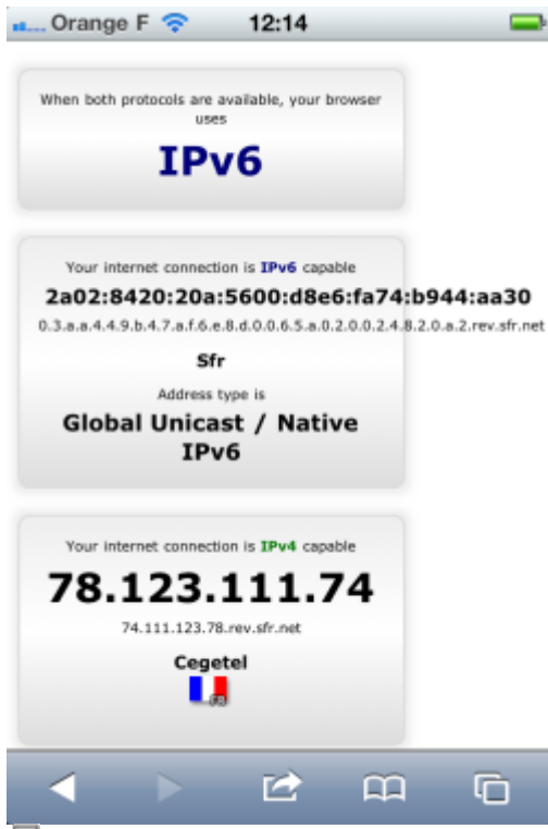
Figure 2. Testing IPv6 on an iPhone
