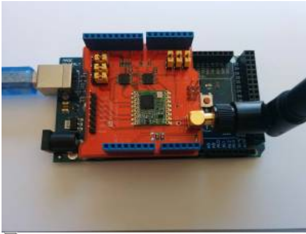
Figure 1. Arduino with LoRa Dragino shield.
