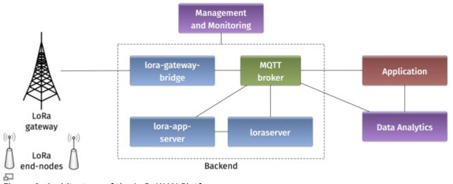
Figure 1. Architecture of the LoRaWAN Platform
