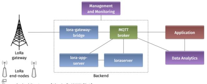
Figure 1. Architecture of the LoRaWAN Platform
