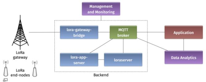
Figure 1. Architecture of the LoRaWAN Platform
