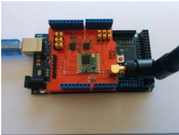
Figure 1. Arduino with LoRa Dragino shield.
