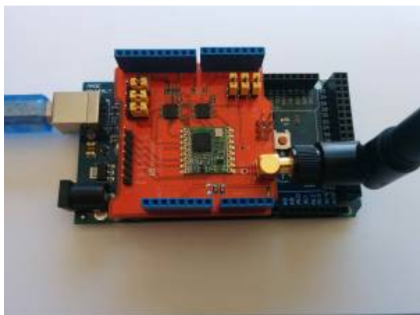
Figure 1. Arduino with LoRa Dragino shield.
