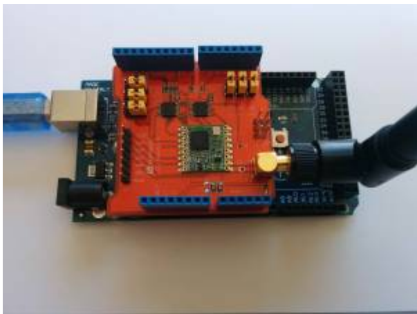
Figure 1. Arduino with LoRa Dragino shield.
