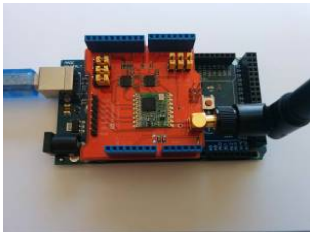
Figure 1. Arduino with LoRa Dragino shield.
