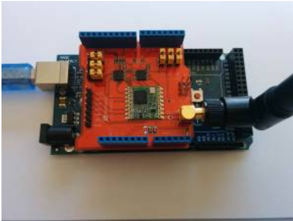
Figure 1. Arduino with LoRa Dragino shield.
