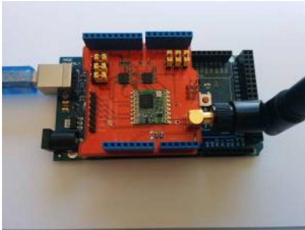
Figure 1. Arduino with LoRa Dragino shield.
