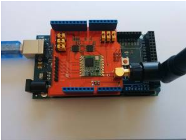
Figure 1. Arduino with LoRa Dragino shield.
