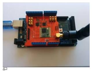
Figure 1. Arduino with LoRa Dragino shield.
