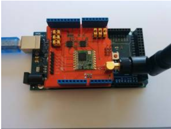
Figure 1. Arduino with LoRa Dragino shield.
