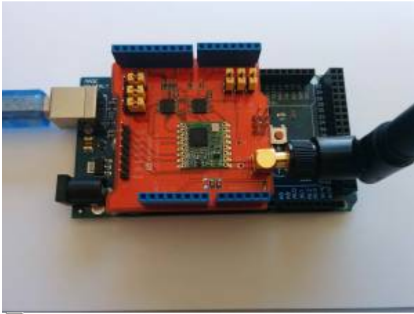
Figure 1. Arduino with LoRa Dragino shield.
