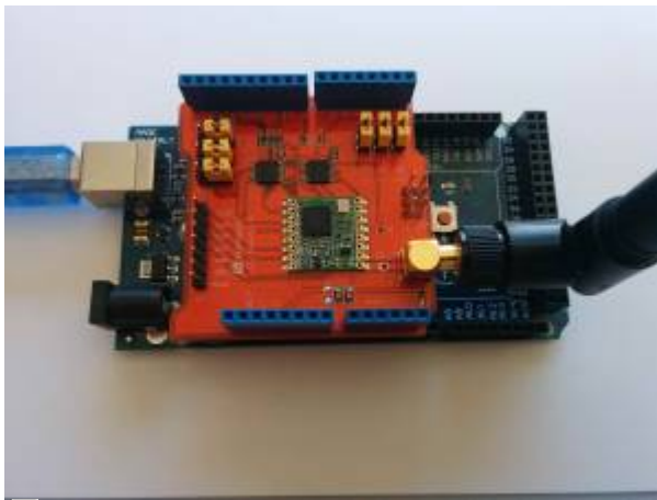
Figure 1. Arduino with LoRa Dragino shield.
