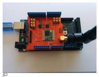
Figure 1. Arduino with LoRa Dragino shield.
