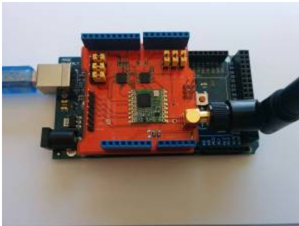
Figure 1. Arduino with LoRa Dragino shield.
