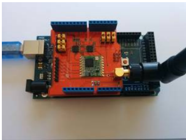
Figure 1. Arduino with LoRa Dragino shield.
