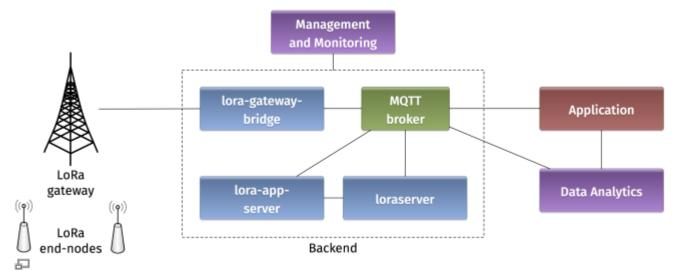
Figure 1. Architecture of the LoRaWAN Platform
